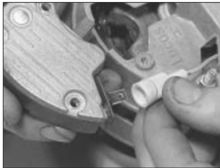
7.7b Disconnecting the field connector (Magnet-Marelli alternator)
