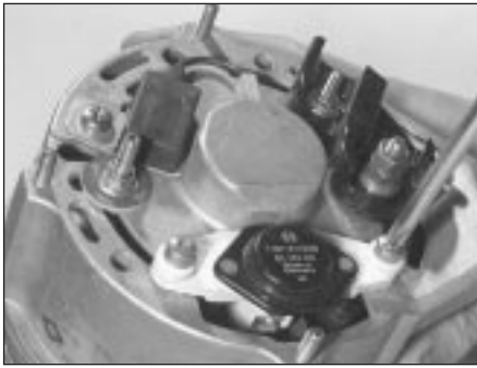
7.3a Undo the retaining screw and . . .
