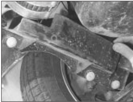
6.3 Removing the drivebelt splash guard (where fitted)
